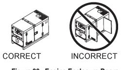
Figure 29. Engine Enclosure Doors
